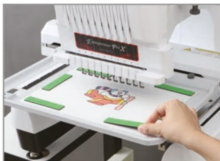
Secure with the magnets
