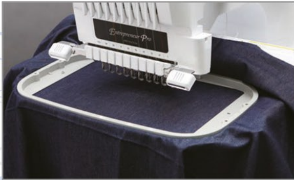
Cloth outside the frame is kept on top of the frame and out of the way
