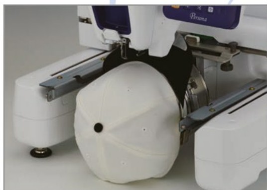
Set completed cap directly onto the machine
